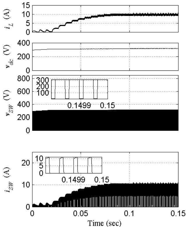
Fig.3 Starting and steady state performance of boost DC-DC converter
