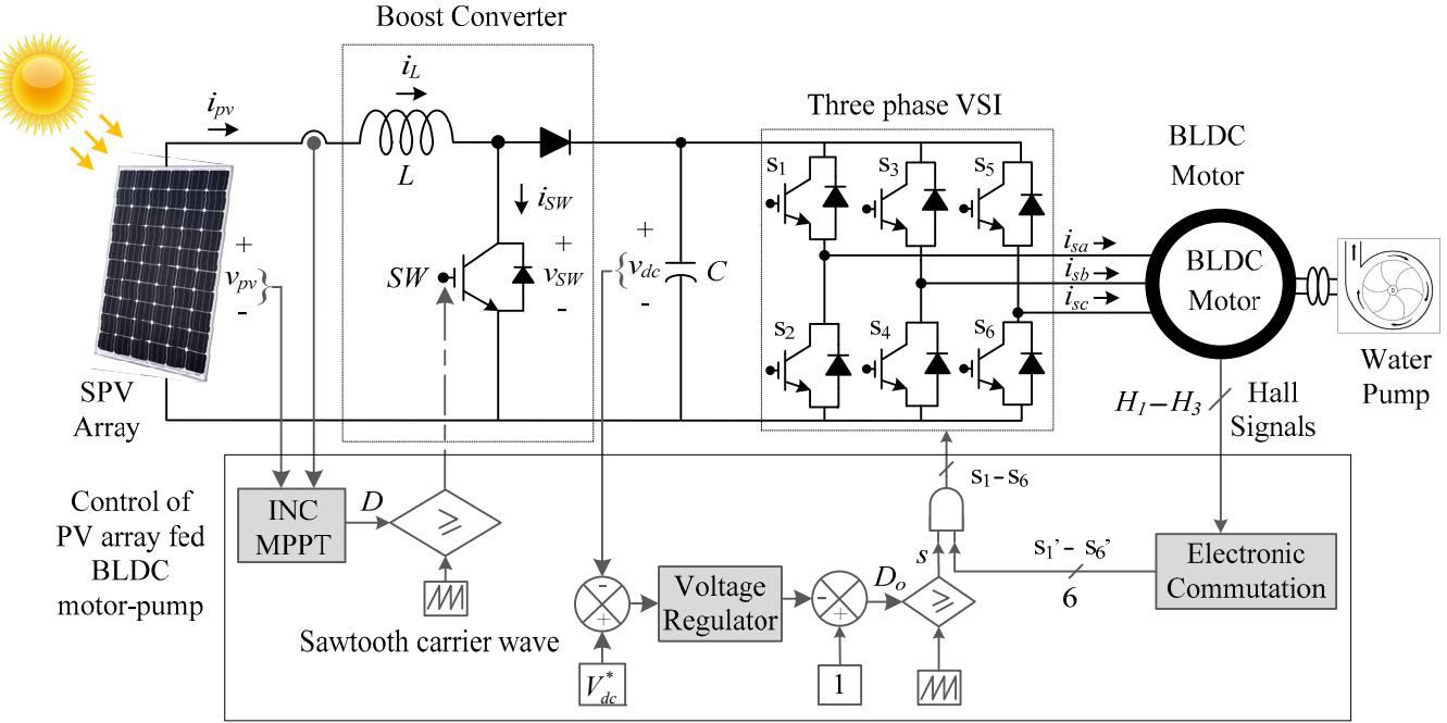
Fig.1 Configuration of PV array fed BLDC motor-pump.
