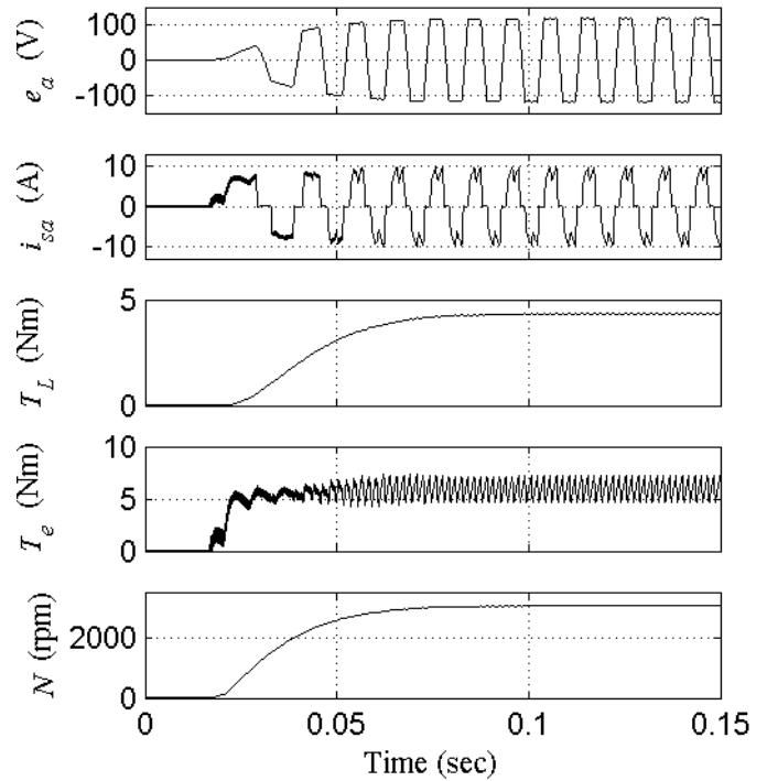
Fig.4 Starting and steady state performance of brushless DC motor-pump
