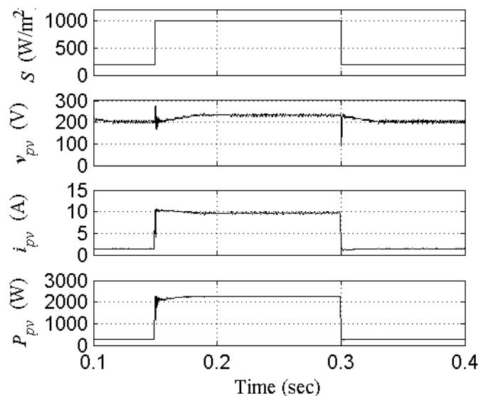
Fig.5 Dynamic performance of solar PV array
