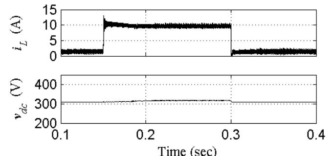
Fig.6 Dynamic performance of boost DC-DC converter
