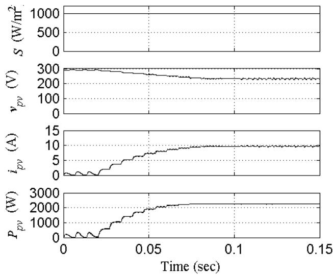
Fig.2 Starting and steady state performances of solar PV array
