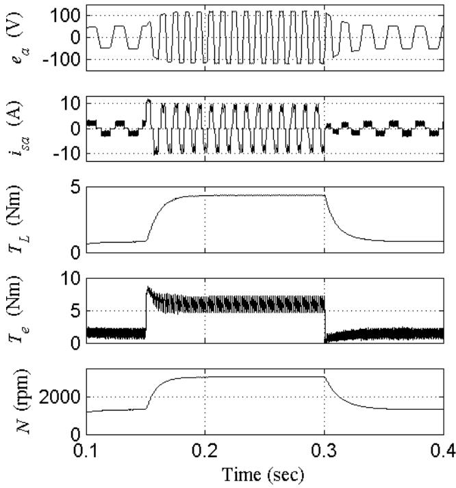
Fig.7 Dynamic performance of brushless DC motor - pump
